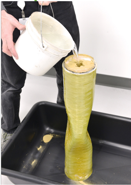
7. Washout Tool with Tap Water
