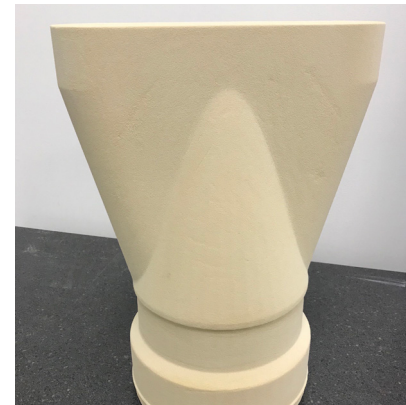
3D Printed Form Before Coating
