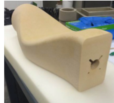
3. Depowder and Clean the Tool Form
