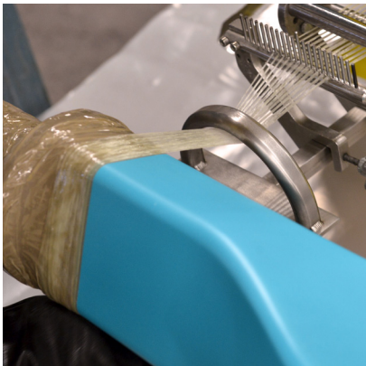
Proprietary Blue Coating Water soluble to 180° Celsius or 356° Fahrenheit
