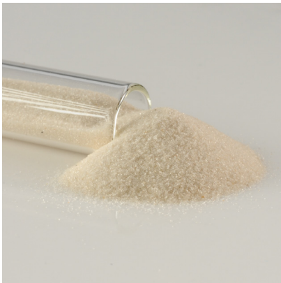
Silica Sand CTE 20 ppm/°C (11 ppm/°F)
