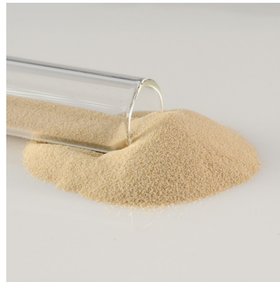
Ceramic Sand CTE 3 ppm/°C (2 ppm/°F)
