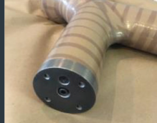
Machined metallic hardware integrated into mandrel for composite winding.
